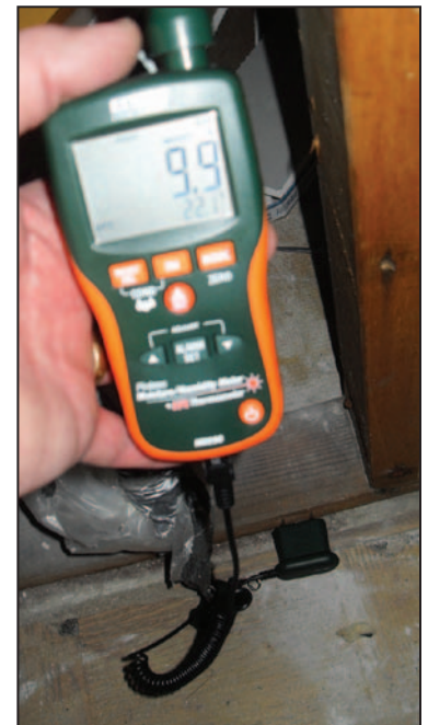
Figure 5: Use of a penetrating (pin-type) moisture meter to verify that wood frame has a water content of less than 15 percent
