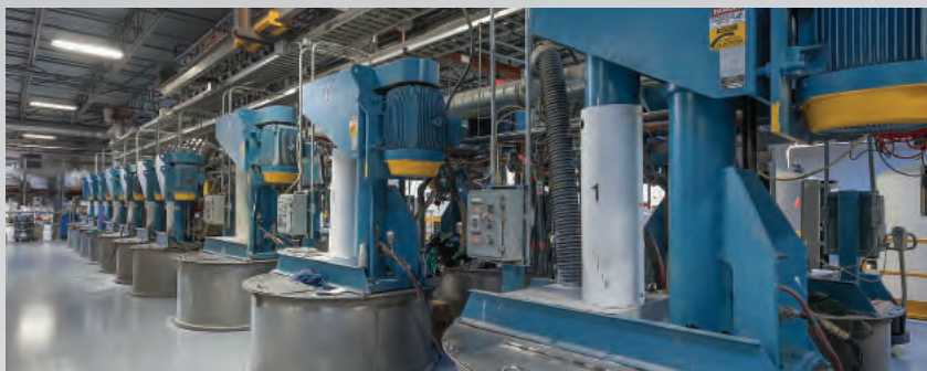
Computer controlled mixing tanks
