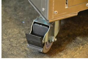
2. Facing the side of the unit, push lever to the right to unlock the handles. Do this on all 4 sides.
