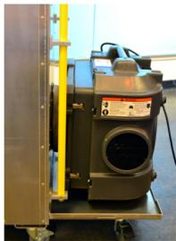
Part B: Attaching negative air machine on the inside of the unit:
