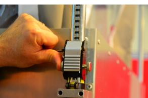
3. Using both hands, grasp both poles and pull up to extend the height of the unit. Switch from both sides when lifting the poles to keep it even. Extend the poles until they reach the top of the ceiling. The unit can accommodate ceilings from 6.5 to 11 ft. The ceiling foam gasket will ensure a tight seal between ceiling and unit.
