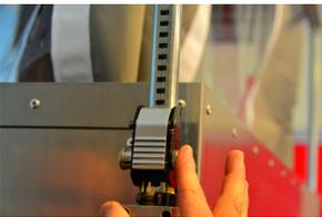
If the unit is being raised by two people, both people should extend the poles on either side at the same time. Make sure that all poles are locked into the support channel at the same level.
