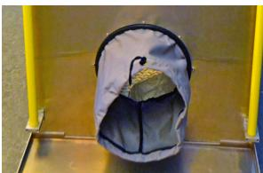
2. Place negative air machine on the AirBase so that both ports are facing each other. Pull port flap over intake manifold on the negative air machine and tighten using drawstrings.
