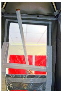
2. Cable pass through: Two white cable pass through ports are located on one side of the unit. These allow cable and wire to be passed through the unit. To open, lift tab at bottom center and then lift flap on front. To close, push flap down and shut tab.
