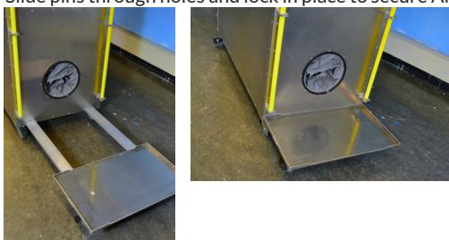
6. Place Kontrol Kube Negative Air Machine on AirBase. (see Section 3 for additional instructions)
