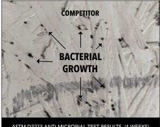
ASTM D3273 ANTI-MICROBIAL TEST RESULTS (4 WEEKS)
