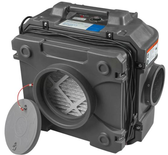
The Kontrol Kube **Complete** Negative Air Machine offers a revolutionary combination of power, efficacy and convenience. Weighing in at 44 lbs this negative air machine delivers a variable speed up to 500 CFM with HEPA filter installed. The Kontrol Kube Complete Negative Air Machine also comes equipped with a DOP Stage 2 First Pass Pre-filter ensure air clearance every time!
