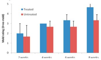
Figure 2. Mold ratings of pine wood samples exposed in the "mold box" test. The treated samples were coated with a sodium carbonate solution according to the directions on the label. Note: The black lines ("error bars") are one standard deviation, which is a measure of variation in the data.
